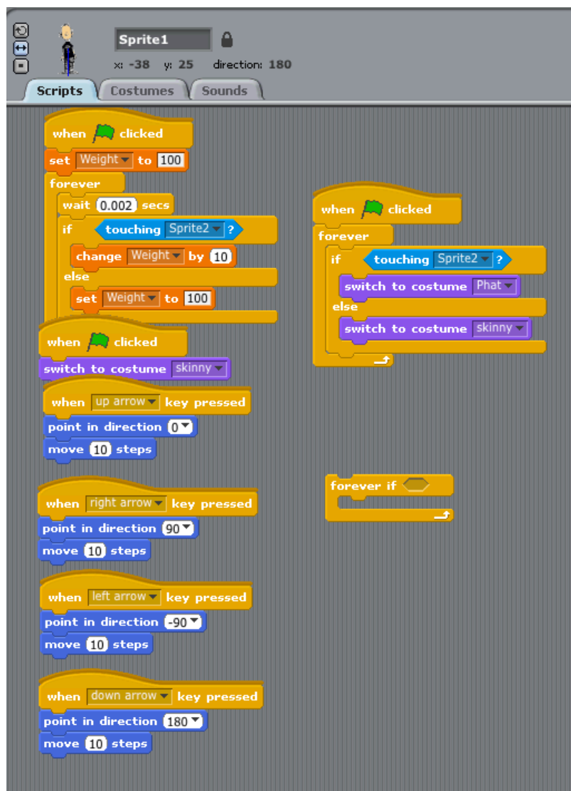
Figure 8.35: Programming script used by Jaime and Eddie to create their “Phat” game.
